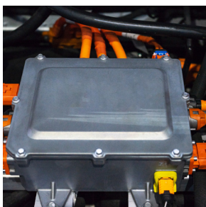
Battery Management System
