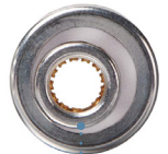
Socket position after self-aligning to the left 1.00mm relative to socket assembly outer housing
